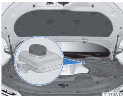
Checking the brake fluid:
