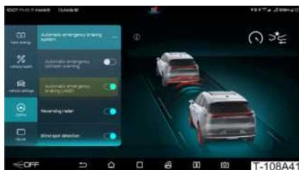
Tap on / > **DiPilot** > **Automatic Emergency Braking System** on the centre console touchscreen to turn **Automatic Emergency Braking (AEB)** on/off.
