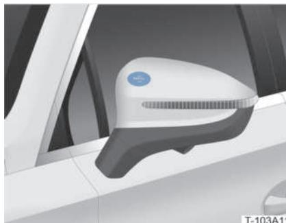
When the vehicle is OFF with all doors and bonnet closed, place the NFC key card on the "NFC" mark on the front left side mirror shell to lock all doors simultaneously. The turning lights flash once, and the side mirrors automatically fold (if the Auto Mirror Fold function is activated).
