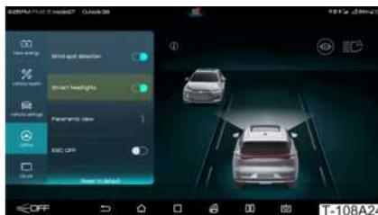
Tap on / > **DiPilot** or pull down **Quick Settings** menu on the centre console touchscreen to turn on **Smart Headlights**.
