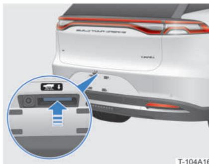
With the vehicle unlocked, press the external boot lid release button to open the boot.
