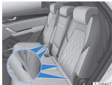
ISOFIX provides anchor points to tightly secure the child safety seat.
