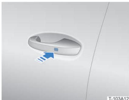
When the 12V battery (starter Fe battery) is in dormant mode, bring the remote control key into the activation area of the front left door, double press the microswitch on the handle to awaken the 12V battery (starter Fe battery), unlock the vehicle and use it normally.
