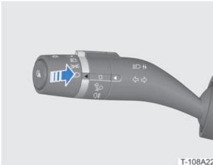
Pull the light stalk switch towards the steering wheel to send an overtaking signal. Release the switch to let it automatically return to its original position. To indicate overtaking intention, pull it repeatedly to flash the high beam.
