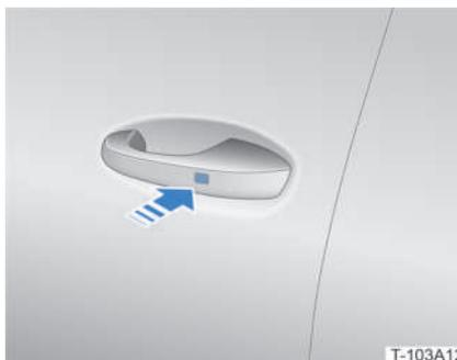
The microswitch can be used when the vehicle is off, and all the doors and bonnet are closed. Walk to the front left/right door activation area with the remote key and:
