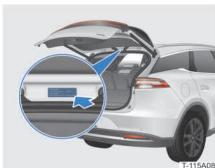
The model and number labels for the rear drive motor are pasted on the boot lid.
