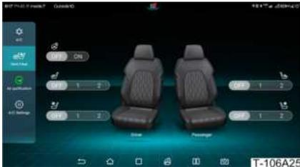
To turn the heating/ventilation function on/off, pull down the **Quick Settings** menu or tap on the
