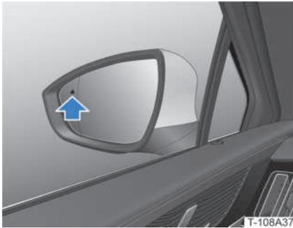
When the radar sensors detect that there is a vehicle in the blind spot of a side mirror when the vehicle is moving at a speed above 30 km/h, the alarm indicator on the corresponding side mirror will light up. If the turning light on the same side is turned on at this time, the warning indicator on the corresponding side mirror will flash, alerting the driver of possible danger if they insist on changing lanes.
