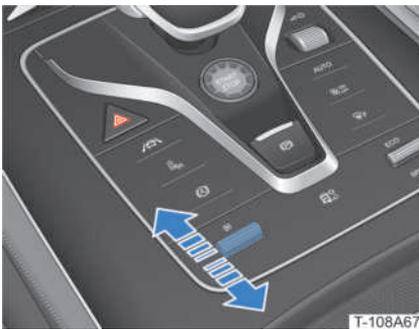
When the vehicle is powered on, push or pull the energy regeneration lever to select the larger or standard regenerative braking
