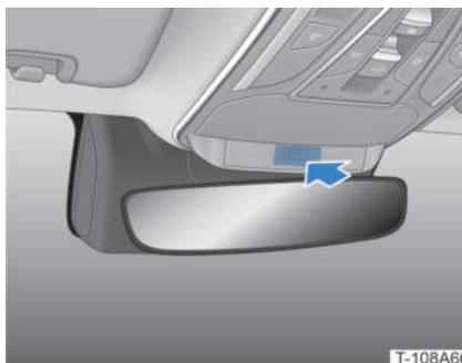
The in-vehicle camera is used for some apps whenever they need to be called via the centre console touchscreen. The camera lens cover can be closed when not needed.
