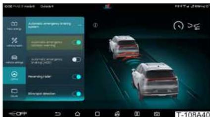
Tap on / > **DiPilot** > **Automatic Emergency Braking System** on the centre console touchscreen to turn **Automatic Emergency Collision Warning** on/off.
