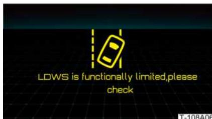
When the vehicle experiences a system fault or operation, the instrument cluster displays the fault/operation prompt information:
