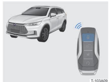
When the vehicle is in anti-theft mode and within the range of the remote control key signal, press the lock button
