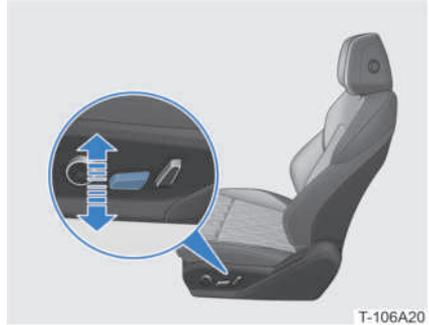
**Cushion adjustment:** toggle the front part of the driver seat position lever up and down to adjust the radian of the seat cushion.
