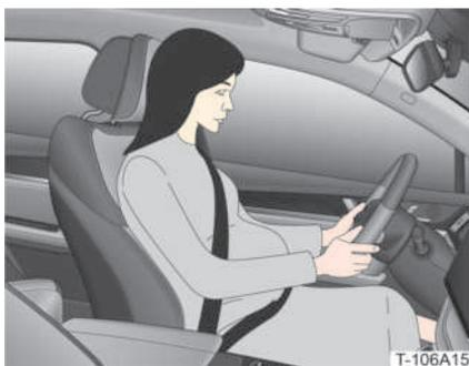
Slowly and smoothly pull out the seat belt from the retractor, cross over the chest and hips. Ensure that the lap portion of the seat belt is as low as possible. Never fasten the lap portion over the abdominal area.
