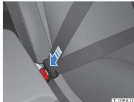
3. Pull the seat belt in the opposite direction and confirm that it has been successfully locked.
