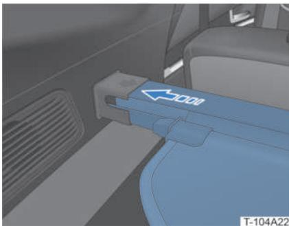
Push in one side of the cover assembly and remove it.
