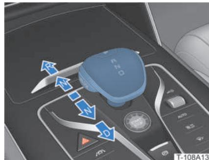
Press the brake pedal, push the gear shift lever in the desired direction after the vehicle has come to a complete stop. After the gear shift lever is released, it automatically returns to the central position.
