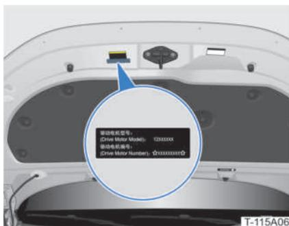
The model and number labels for the front drive motor are pasted on the inner side of the bonnet.
