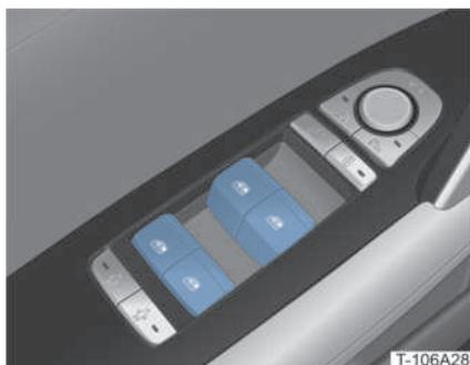
Window controls are enabled when vehicle is powered ON.
