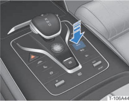
Press the "AUTO" button or tap on the "AUTO" button on the Climate Controls of the centre console touchscreen to enter auto control mode.
