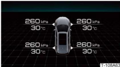
If no tyre pressure fault is displayed on the instrument cluster, the tyre pressure information can be accessed on the instrument cluster menu - driving information. Tyre pressure information includes:
