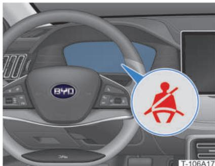
The vehicle is equipped with a seat belt sound reminder.
