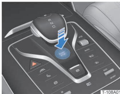
With the remote control key inside the vehicle, press the brake pedal and SRART/STOP button to power on/off the vehicle.
