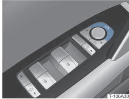
When the vehicle is powered on, press the
