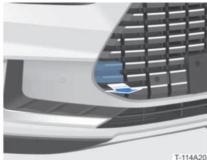
3. Insert the towing hook into the towing hole, rotate it clockwise and tighten it.
