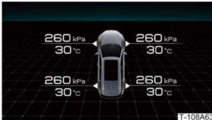
If no tyre pressure fault is displayed on the instrument cluster, the tyre pressure information can be accessed on the instrument cluster menu - driving information. Tyre pressure information includes:
