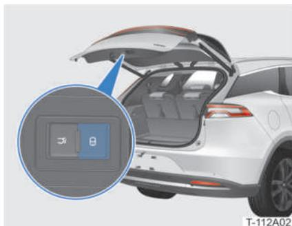
When the vehicle is OFF with the boot opened, but all doors and bonnet closed, walk to the boot carrying the remote control key and press the
