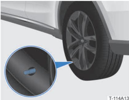
2. Screw the inflator pump connector onto the tyre valve. A slight air leakage sound will be heard from the valve, indicating that the air is circulated. Continue screwing until there is no air leakage sound.
