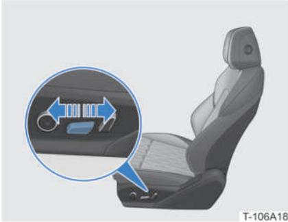
**Forward/backward adjustment:** move the position lever back and forth to slide the seat forward or backward.
