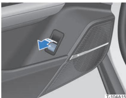
When the boot is closed, pull the interior boot switch
