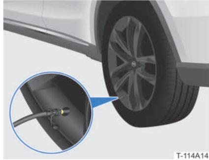
3. Plug the power plug into the on-board power supply port.
