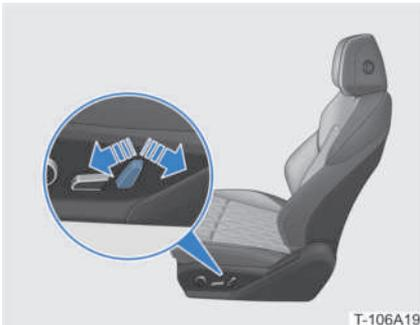
**Backrest adjustment:** toggle the backrest adjustment lever to adjust the backrest angle.
