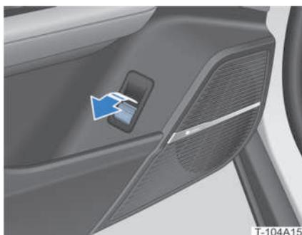
When the boot is closed, pull the interior boot switch
