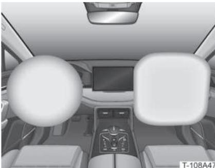
The front seat airbags are installed in the steering wheel and dashboard panel, and
