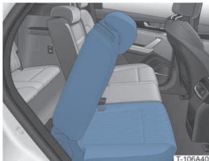
3. Slide the seat back and pull its backrest to its locked position.
