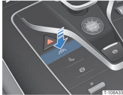
Press the LKS button
