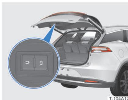
When the boot is open, press the close button
