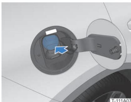
3. Insert the charging connector into the charging port.
