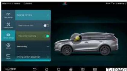
The **Auto-Tilt** feature can be turned on/off when the vehicle is powered on by tapping on / > **Vehicle Settings** > **Side Mirror Auto-Tilt** on the centre console touchscreen.
