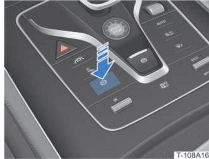
After the conditions above are all met, press the AVH button to turn AVH on. The switch indicator then lights up. At this time, the AVH function is in standby, and the AVH indicator on the instrument cluster lights up (white).
