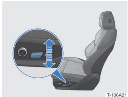
**Height adjustment:** toggle the rear part of the driver seat position lever up and down to adjust the height of the seat cushion.
