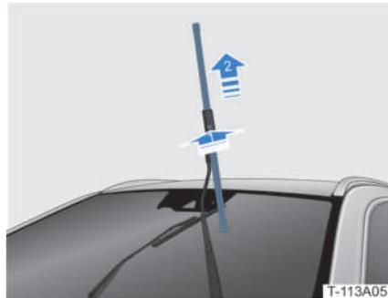
5. Follow the same procedure in reverse to insert the new wiper blade into the wiper arm and lock it in place.
