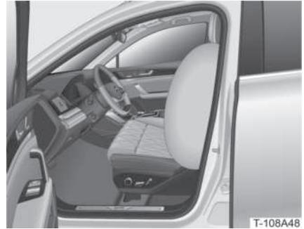
The front seat side airbags are installed on the side of the driver and front passenger seat backrests, and are marked with the lettering "AIRBAG".
