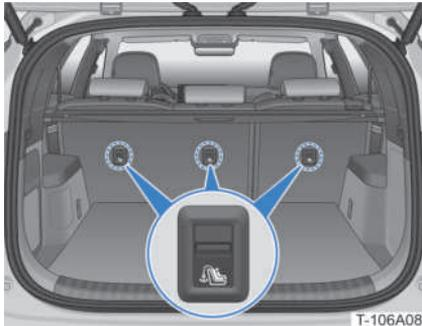
LATCH provides tether anchors to secure a child safety seat flexibly.
