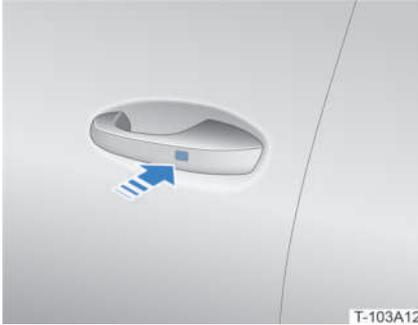
The Microswitch on the front door handles operates when the vehicle is locked, powered off, and the remote control key is within the front doors activation range:
