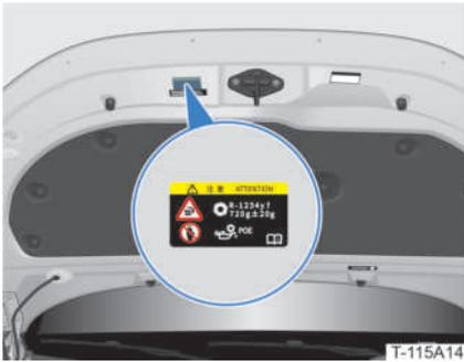
Refrigerant Refill and Cooling Fan Warning Labels
