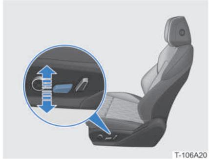
**Cushion adjustment:** toggle the front part of the driver seat position lever up and down to adjust the radius of the seat cushion.
