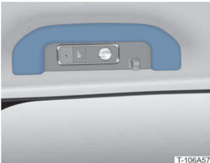
Passengers can maintain their balance by holding on to the roof handles while riding. The handles return to their original position once released.
