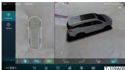
Tap on the
