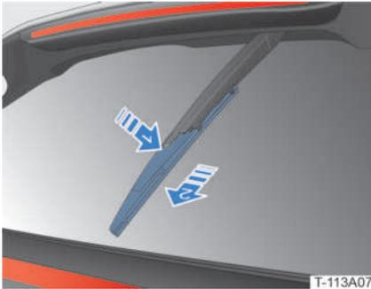
5. Follow the same procedure in reverse to install the new wiper blade, and gently lay the wiper arm onto the rear windscreen.
