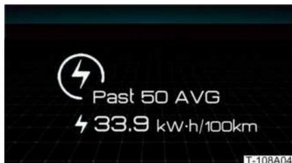
When there is no fault/operation prompt information on the instrument cluster, roll the right roller to select the "Driving Information" interface.
