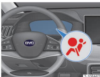
When the vehicle is powered on, the system will conduct a self-inspection. The SRS fault warning indicator will light up for a few seconds and then automatically go out, indicating that SRS is functional. If the fault
