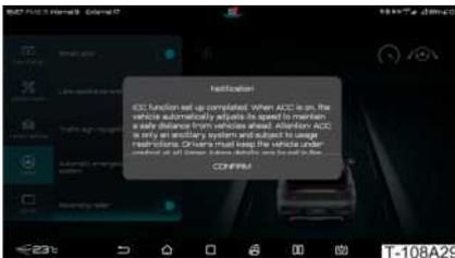
Tap on / > **DiPilot** or pull down **Quick Settings** menu on the centre console touchscreen to turn **Smart Pilot** on along with a prompt popping up on the screen.
