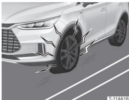
If a tyre bursts or leaks while driving, hold the steering wheel tightly with both hands and try to keep it from steering on its own. Press the brake pedal lightly to slow down, so that the vehicle can continue moving straight. Drive slowly to a safe area and stop. Replace the tyre or contact any rescue service as needed.
