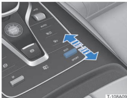
Move the adjustment lever forward to enter ECO mode.
