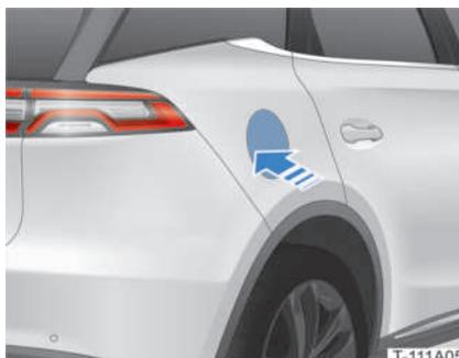
The charging port is located at the rear right of the vehicle.
