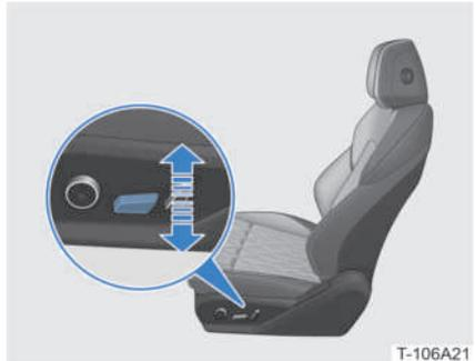
**Height adjustment:** toggle the rear part of the driver seat position lever up and down to adjust the height of the seat cushion.
